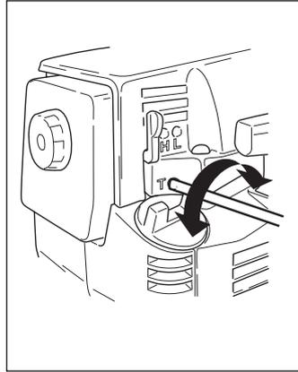
**CAUTION!** Contact your servicing dealer, if the idle speed setting cannot be adjusted so that the cutting attachment stops. Do not use the machine until it has been properly adjusted or repaired.
