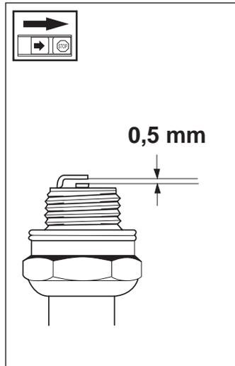
**If the machine is low on power, difficult to start or runs poorly while idling always check the spark plug first before taking any other action.**
